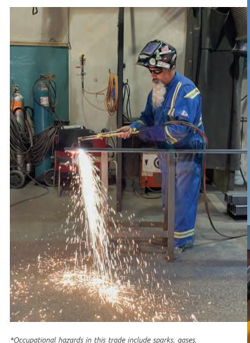
hazardous fumes, burns, heavy lifting, exposure to ultraviolet light and infra-red rays, working at heights, working in confined spaces, and in trenches.
